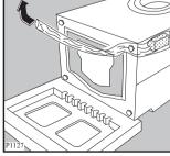
5. Set the machine upright and remove the remaining rear screw. Slide out the relevant pin.
